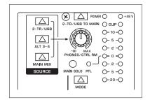
Fig. 2.11: Control room/phones section, level meter
